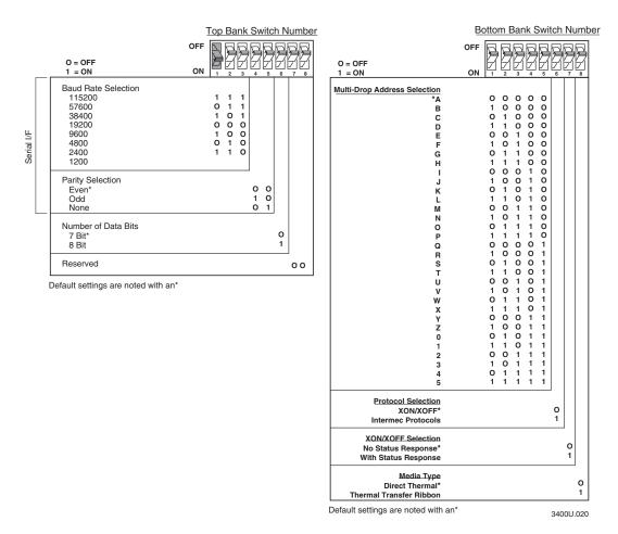
**DIP switch settings:** These charts illustrate the settings for the DIP switches on the top and bottom banks. For a description of each setting, see the DIP Switch Settings Descriptions table on page 12.
